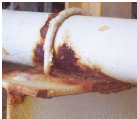
Above, the result of crevice corrosion on a pipe. Trapped moisture has caused substantial wall loss that could result in catastrophic failure.
